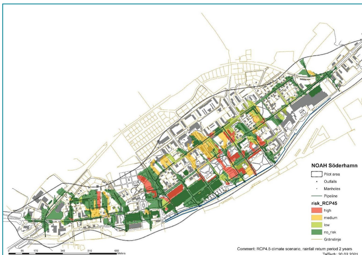
Figure 9. Example of the EWL flood risk map developed for NOAH pilot in Söderhamn, Sweden (RCP 4.5 rainfall period 2 years).
