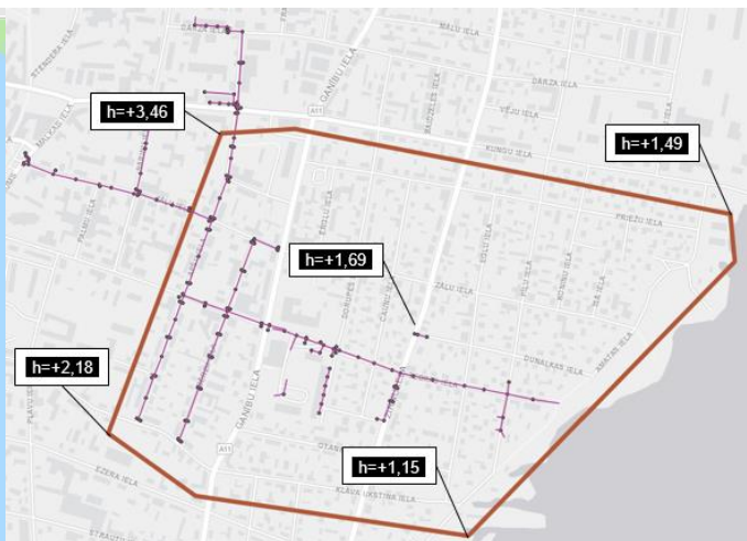
Figure 2-4 Ground elevations in Tebras street catchment area and stormwater pipe layout
