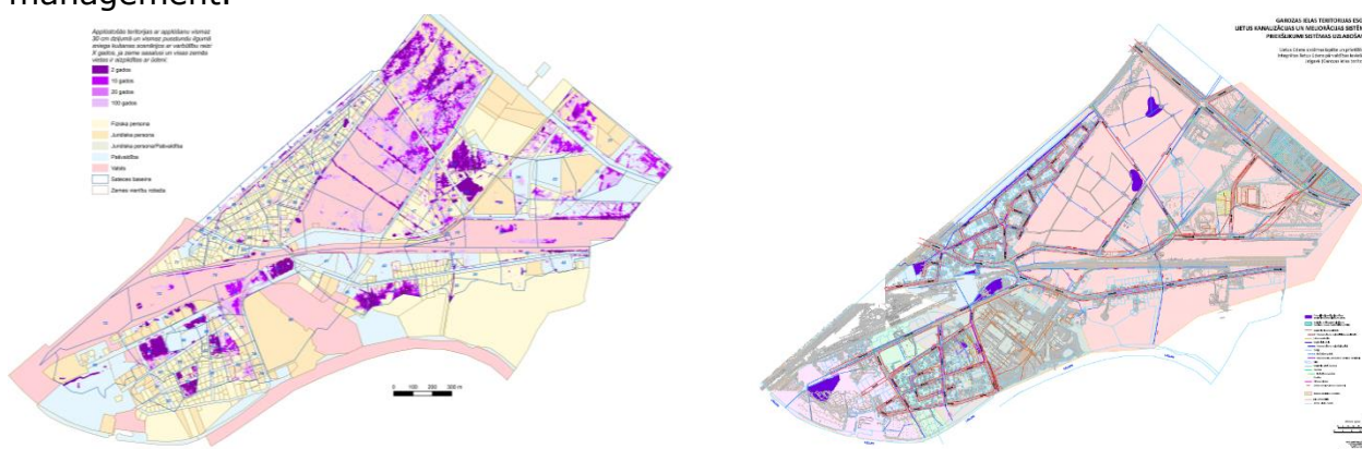
Figure 4 Modelled flood areas (extreme precipitation and snow melt of different probabilities) and proposed flood risk management measures in Garozas Street catchment basin pilot management plan in the city of Jelgava
