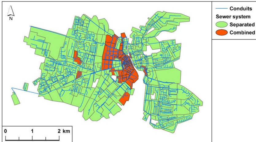
Figure 12. Conduits and catchments simulated in the Słupsk pilot area using SWMM
