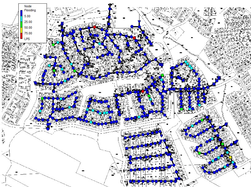
Figure 4. SWMM model result showing the flow from surcharging nodes for an extreme rainfall event.
